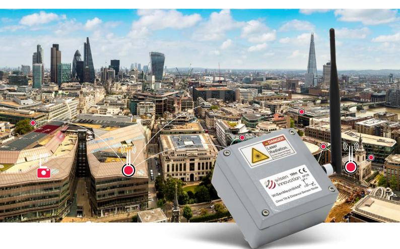
This internally powered sensor node allows measurement of tilt in any axis from a horizontal plane and a distance to any surface up to 100m away without a reflector. With a complete tilt range (360°), high accuracy ( $\pm 0.002^{\circ}$ ) and resolution ( $\pm 0.0001^{\circ}$ ) in addition to distance measurement (005m ~ 100m) with high accuracy ( $\pm 1$ mm) and resolution ( $\pm 0.1$ mm) this sensor is very versatile.
